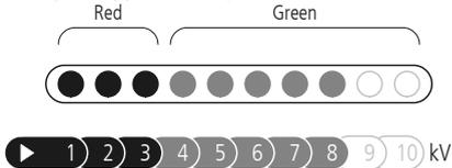
*Note:* If ten Indicator light segments are illuminated, the output voltage may be more than 10 kV (10,000 V).
