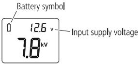
When the voltage is outside the normal range (below 11.8 V or above 17 V), the battery symbol flashes.
